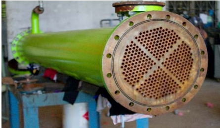
OIL COOLER Clients:- MMGXL Saxon Country:- Cambodia
